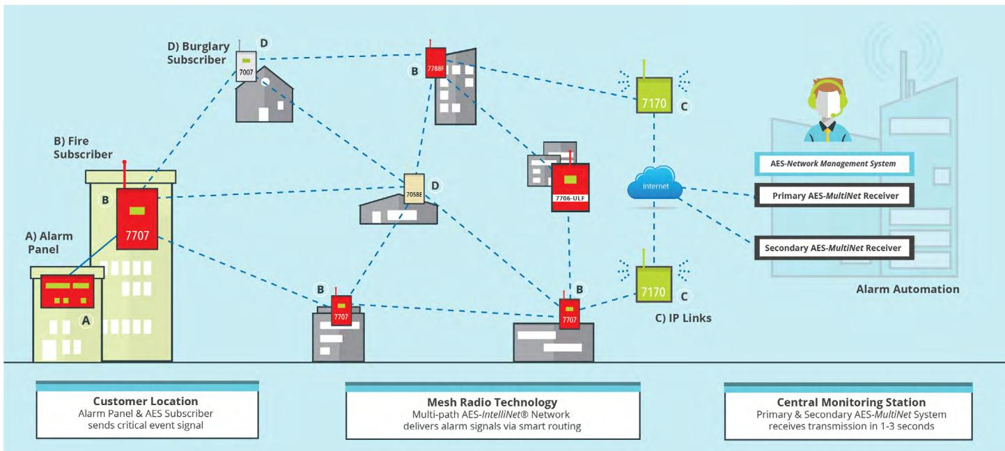
The *IntelliNet 2.0* Fire Subscriber has an 8 Zone modular design for expansion with normal and reverse polarity, POTS and DACT interfaces with an option for the 7794A AES-*IntelliPro* full data module add-on accessory board. AES subscribers' intelligent software automatically detects new hardware and devices to reduce installation time.
